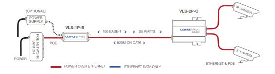
Range is for typical 24AWG Cat5e or 23AWG Cat6, 4-pair UTP.
